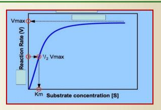
NOTE: The equation describe how reaction velocity varies with substrate concentration.
