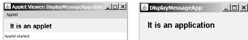
FIGURE 18.8 The DisplayMessageApp class can run as an application and as an applet.
