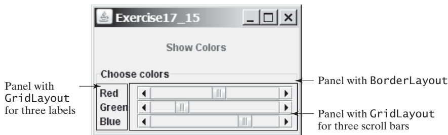
FIGURE 17.46 The foreground color changes in the label as you adjust the scroll bars.
