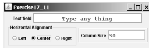
FIGURE 17.42 You can set the horizontal-alignment and column-size properties of a text field dynamically.
