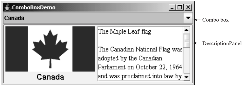
FIGURE 17.22 A country's info, including a flag image and a description of the flag, is displayed when the country is selected in the combo box.
