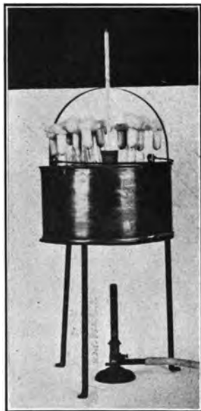
FIG. 13.—Water-bath for Melting Agar or Gelatin for Plating, containing a Removable Copper Test Tube Rack. (Orig. Northrup.)
