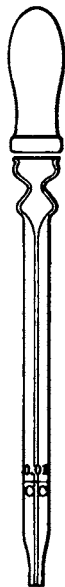
FIG. 58.—Capillary Pipette used in the Microscopic Method for Counting Bacteria in Milk. Note the straight narrow bore and the square tip.
