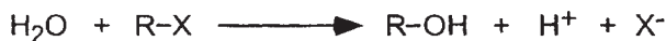
Figure 8.3 Model reactions for hydrolysis of acid derivatives and halogenated organics, where R and R' = C or H; Y = O, NR, or S; Z = C, P, or S; and X = halogen.
