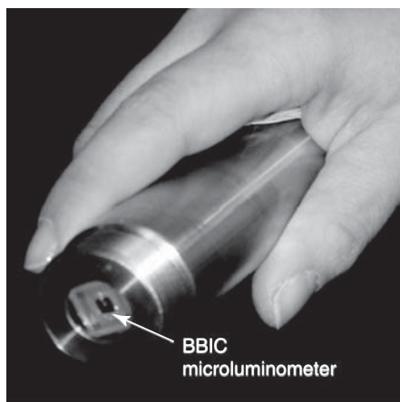
Figure 9.9 BBIC microluminometer, here incorporated into a handheld probe; permits unattended monitoring of bioluminescence from adhered whole-cell lux -based bioreporters.
